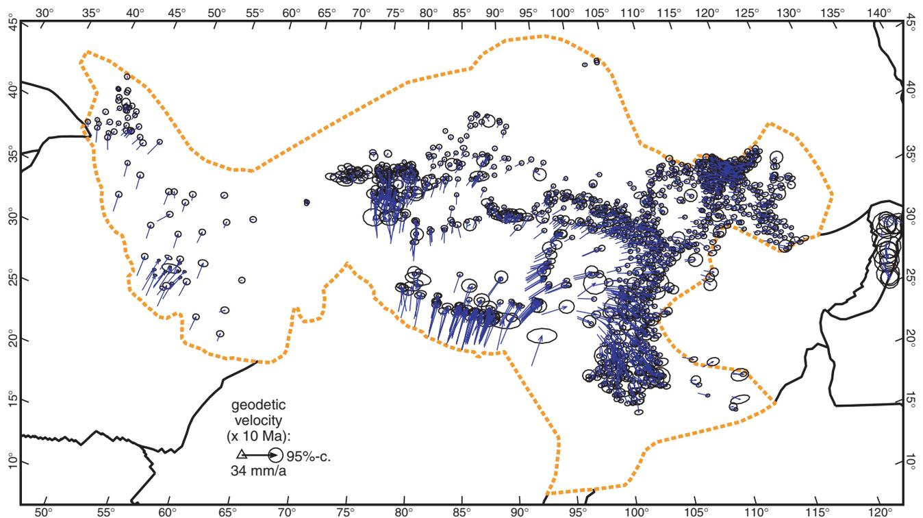
**Figure 3.** Relative horizontal velocities of geodetic benchmarks in the Persia–Tibet–Burma orogen. Geodetic data are compiled from various sources listed in text. All geodetic benchmark velocities are in the Eurasia reference frame. Plotted velocity vectors are projected displacements during 10 million years. Ellipses show 95 per cent confidence limits.
