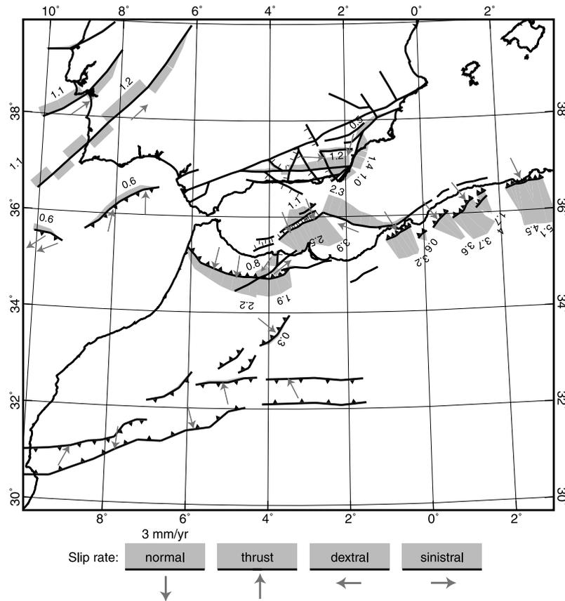
**Figure 7.** Fault slip rates ( $\text{mm yr}^{-1}$ ) obtained with the fault network of model set 1 and a fault friction coefficient  $f_f = 0.05$ . Small gray arrows in hanging walls show the directions of slip. Unlabeled faults have slip rates so low that they are probably numerical artifacts and should be considered as inactive.
